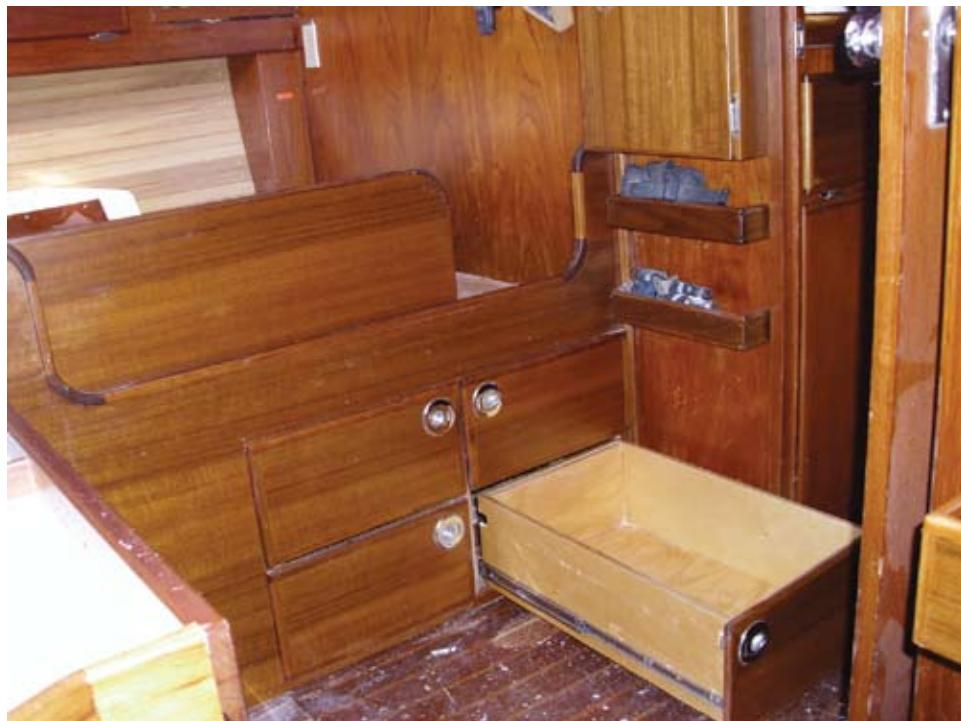
The drawers under the Pullman berth were impractically deep, had to be lifted to open and were difficult to slide on their wooden tracks. Replacing the two deep drawers with four new drawers on stainless steel full-extension slides created 25% more space, all of which was more usable. The slam latches provide secure closure and perfect handles for easily pulling the long drawers open. These drawers will receive cedar liners before we set sail.
