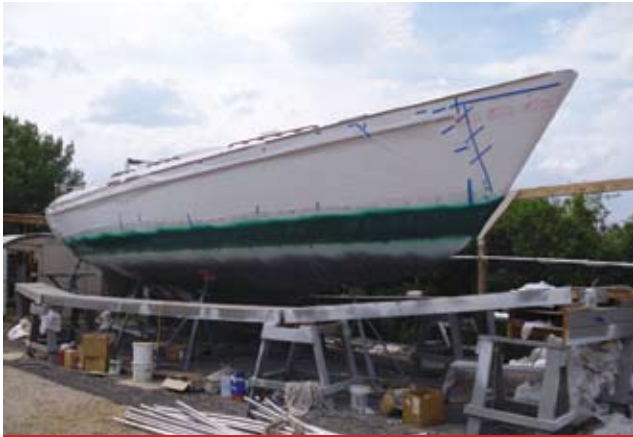
Top, the hull was masked while the boot stripe was sprayed. Bottom, Alex and Pete conduct a tack rag wipe and inspection prior to spraying the topcoat
