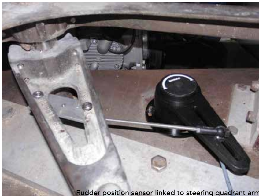
Rudder position sensor linked to steering quadrant arm
