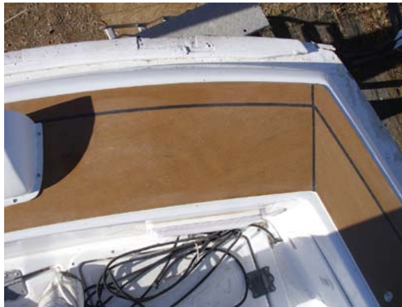
This page, PlasTEAK pattern placed, then applied to the coaming. Opposite, PlasTEAK on the toe and rub rails
