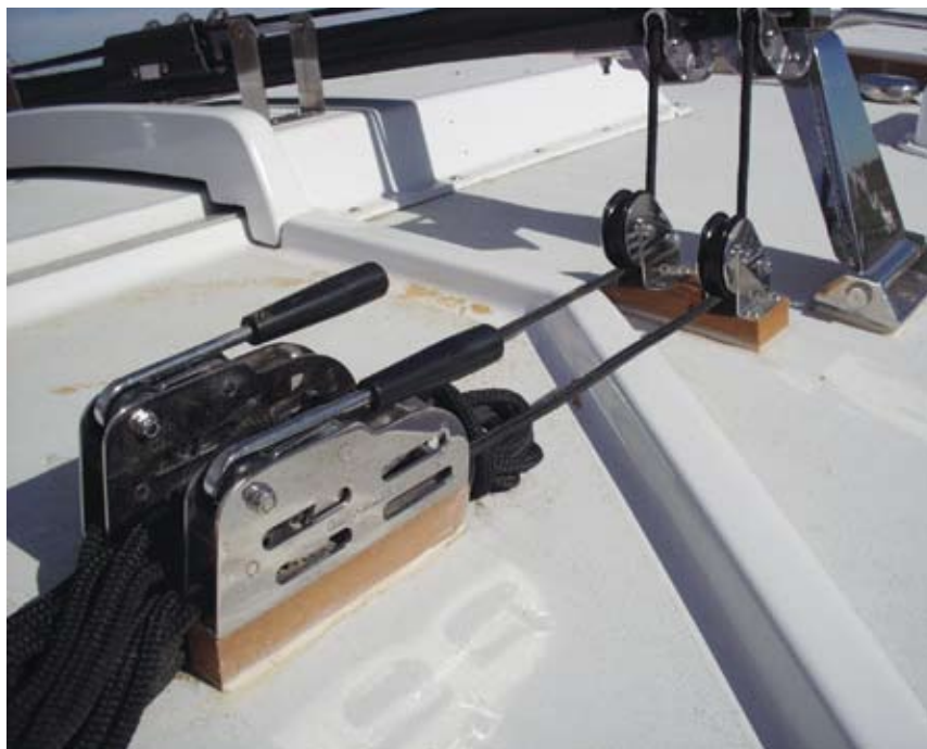
Left, PlasTEAK blocks under Garhauer rigging to the traveler. Bottom, thruhull hole-shaping tools
