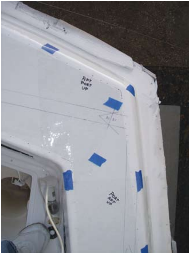
This page, PlasTEAK pattern placed, then applied to the coaming. Opposite, PlasTEAK on the toe and rub rails
