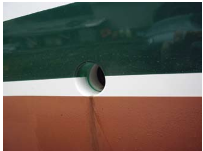
Clockwise from top left: plumbing parts; the old mushroom partially ground away; the clean look of flush thruhulls
