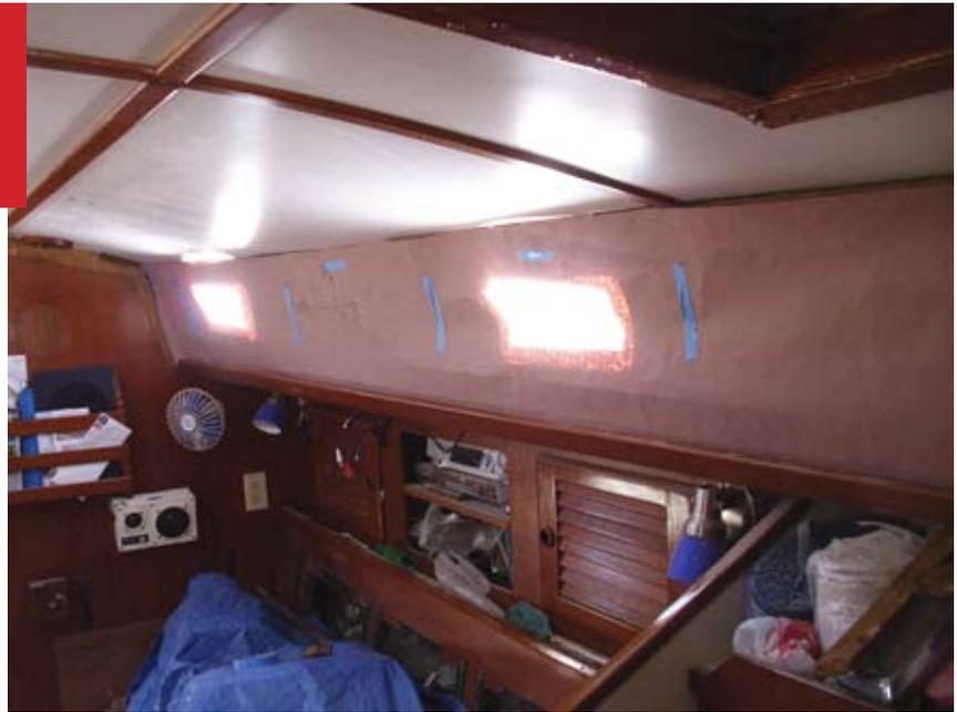
out removing a port. For boats with fairly thin cabin topsides, as is the case with our Pearson, a teak spacer must be added on the inside of the cabin. New Found also provides precise length screws in 3 to 5mm increments for each port.
